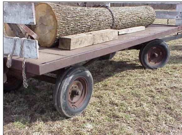
Pneumatic tires provide a large bearing surface and cushion the impact of stones and other obstructions.
